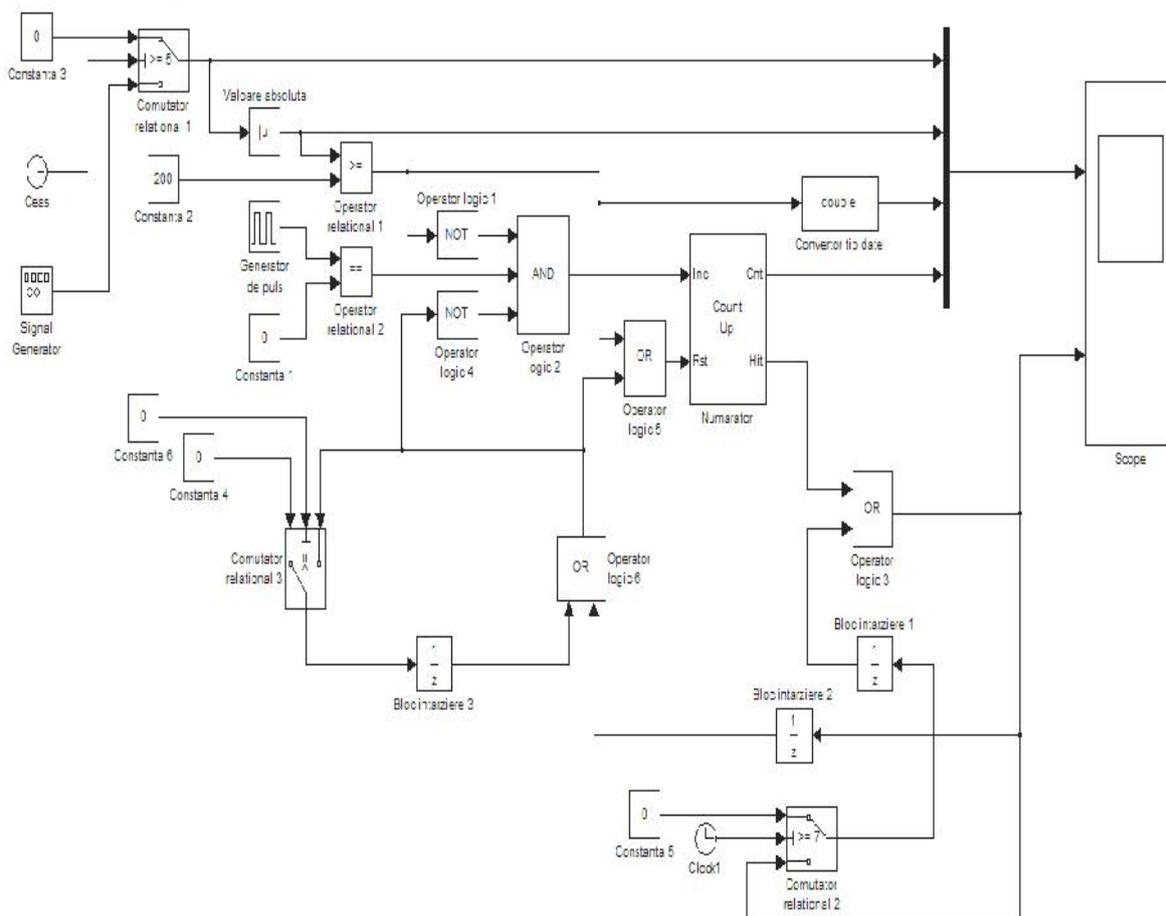
Figure 1. SIMULINK model of the static switch.
