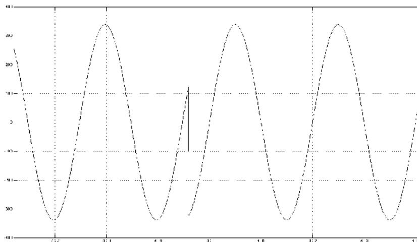
Figure 6. The switch between the two sinusoidal voltage sources.
